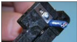
Score cable with stripper CAT. NO. 45-165
