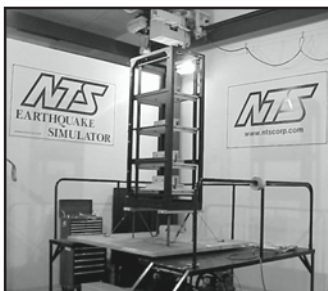
Seismic testing of the Raised Floor Kit. PART# AFSB18, cabinet sold separately
