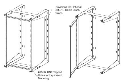
**Receiving, Unpacking, and Removing the SRD Swing Rack** Inspect and report damage before receiving. Unpack the SRD Swing Rack by carefully removing the corrugated cartons and corners. Avoid damaging the SRD Swing Rack when removing packaging.
