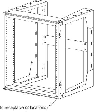
Secure retractable pins into receptacle (2 locations)
