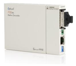
This Gigabit Ethernet to MM Fiber Media Converter creates a cost-effective Gigabit Ethernet-fiber link, transparently converting to/from 1000BaseT Ethernet signals and 1000BaseSX optical signals to extend an Ethernet network connection over a multimode fiber backbone.
