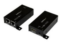
The ST121SHD30 HDMl® over CAT5e/CAT6 Video Extender kit lets you extend HDMl audio/video and an IR remote control signal by up to 100 feet (30 Meters) over dual Cat5e or Cat6 cable. For added versatility this HDMl extender kit is powered via the HDMl bus, and does not require any additional power adapter.
