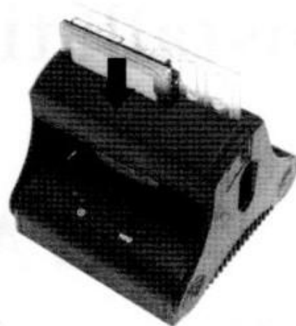
4) Insert 2.5" hard drive plastic fixture
