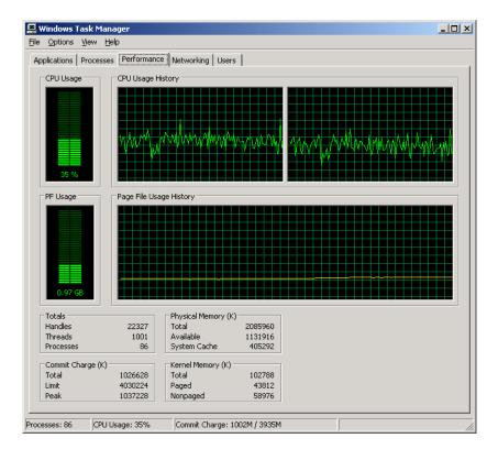
As you can see in the Task Manager screen capture, processor utilization was well below 40% and the available memory was 1.1 GB of the 2 GB installed. This clearly shows that the Dell system had plenty of performance to handle this configuration.
