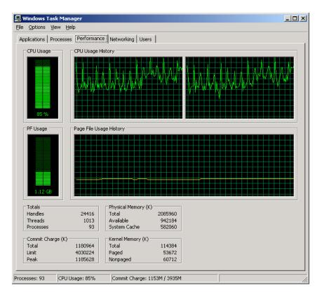
In this expanded application environment, average processor utilization is about 85% and the available memory was still 0.9 GB of the 2 GB installed.
